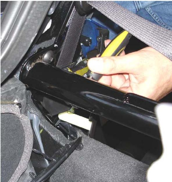
14. Reinstall the trim panels on the rear of the door openings.
