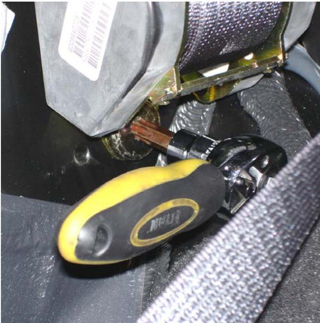
10. Place the Sharkbar B-pillar bracket in place and insert the bolt through the shoulder harness guide and then the bracket. Start the bolt, but do not tighten
