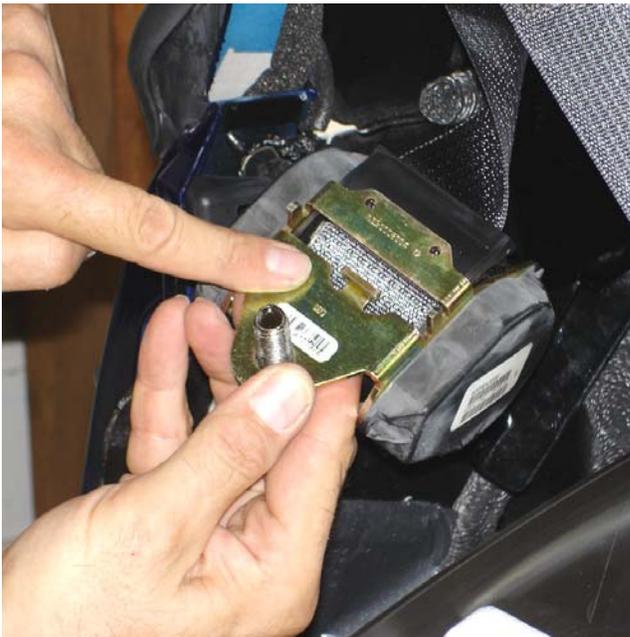
11. Using a 5/16" Allen socket, remove the bolts from the Shark Bar bracket.
