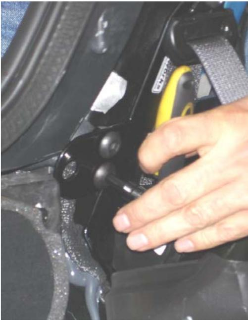
12. If using existing quarter panels locate and drill the holes for the Sharkbar with the provided Template.
